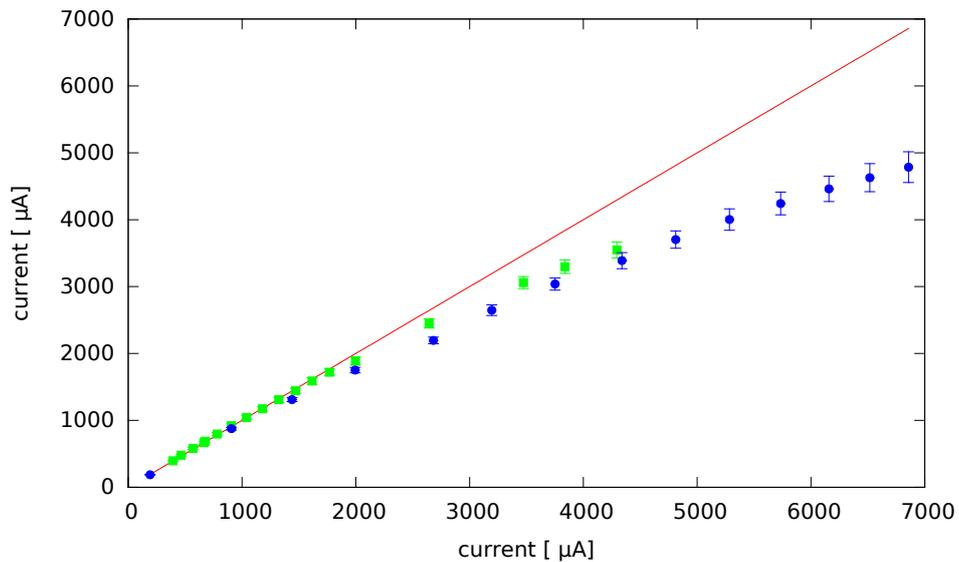
Figure 6: Output of ASC-II detectors, using old board (blue), and new board (green)
