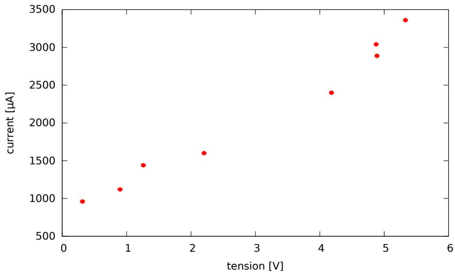
Figure 5: Output current ( $\mu\text{A}$ ) in function of input tension (V) for amplifier of current
